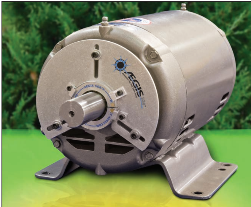
The AEGIS SGR Bearing Protection Ring is available for any size NEMA or IEC motor and comes with a mounting adaptor for fast, easy installation on motors with shaft shoulders, slingers, or other end-bell protrusions.
